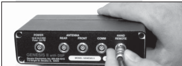
Figure 2.2b Align the red dot on the connector with the red dot on the computer receptacle.
