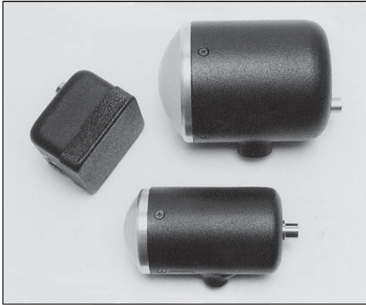
Figure 5 Antennas for the Genesis-II include (clockwise from top right) the K-band silver ring (top) and Ka-band silver ring (bottom) and the Ka-band patch (left).
