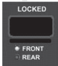
Figure 3.2b When the FRONT light illuminates, the FRONT antenna is transmitting.
